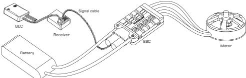
\*Please ensure all solder joints are insulated with heat shrink where necessary All pictures are for reference only
